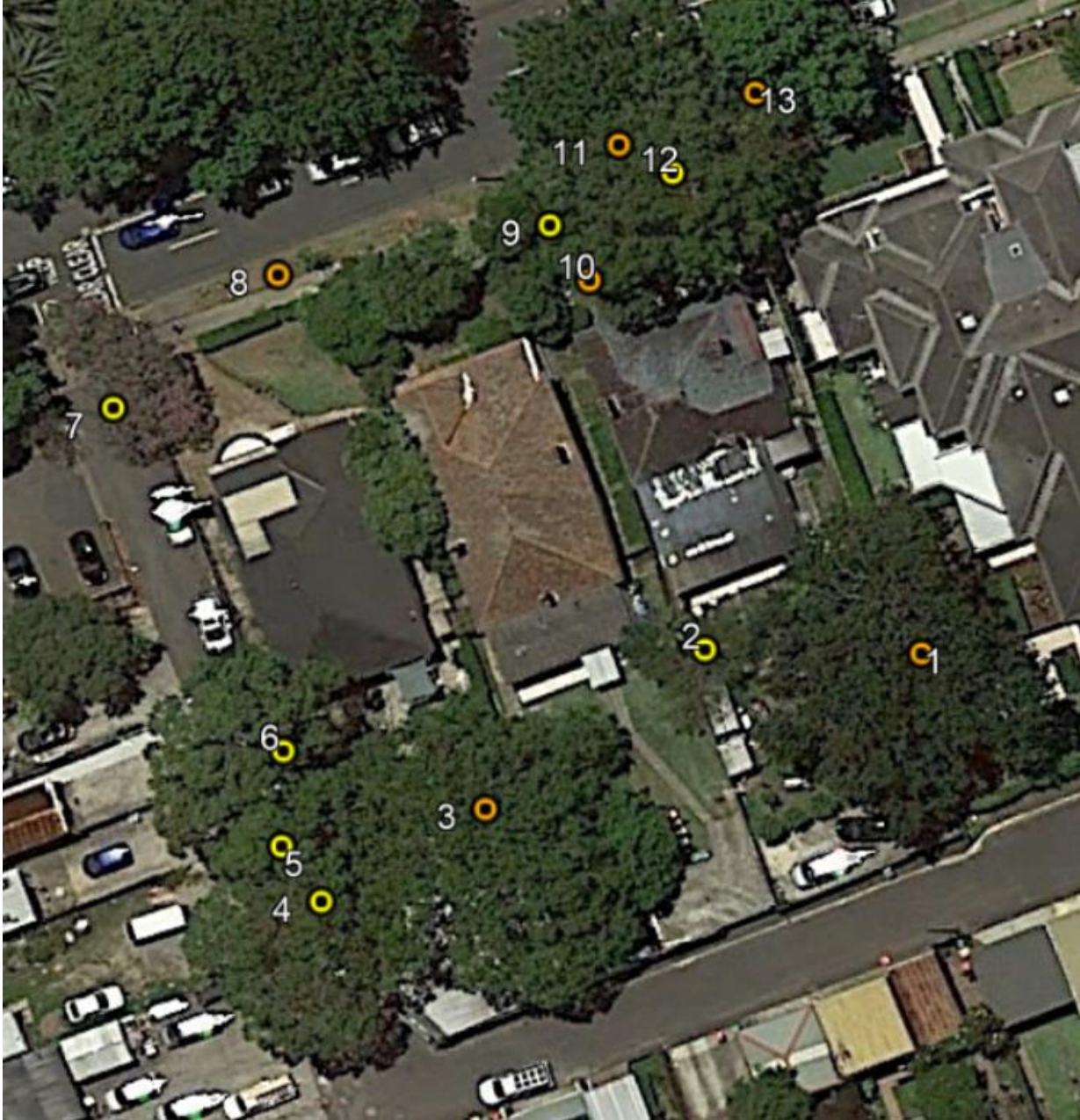
Figure 3- An initial site survey has been completed with the trees located with a Trimble Geo-7x data logger as shown above. Medium retention trees are shown in orange, low retention trees are shown in yellowImage is a clipped KMZ file from Google Earth. 5
